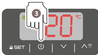
encendido/apagado panel activation/deactivation of the control panel
