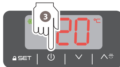
encendido/apagado panel activation/deactivation of the control panel
